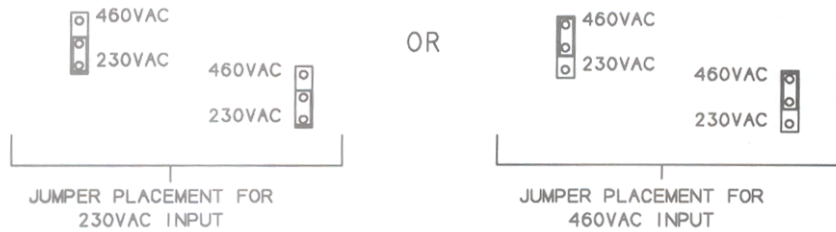
Figure 9 Input Voltage Mini-Jumpers Placement For 230VAC or 460VAC Operation
