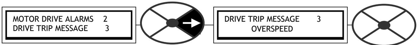
If the speed feedback signal exceeds 110% of rated speed for longer than the alarm delay time, then the overspeed alarm is activated. This alarm is likely to be caused by a badly adjusted speed loop or overhauling of motors controlled by 2 Quadrant models.
