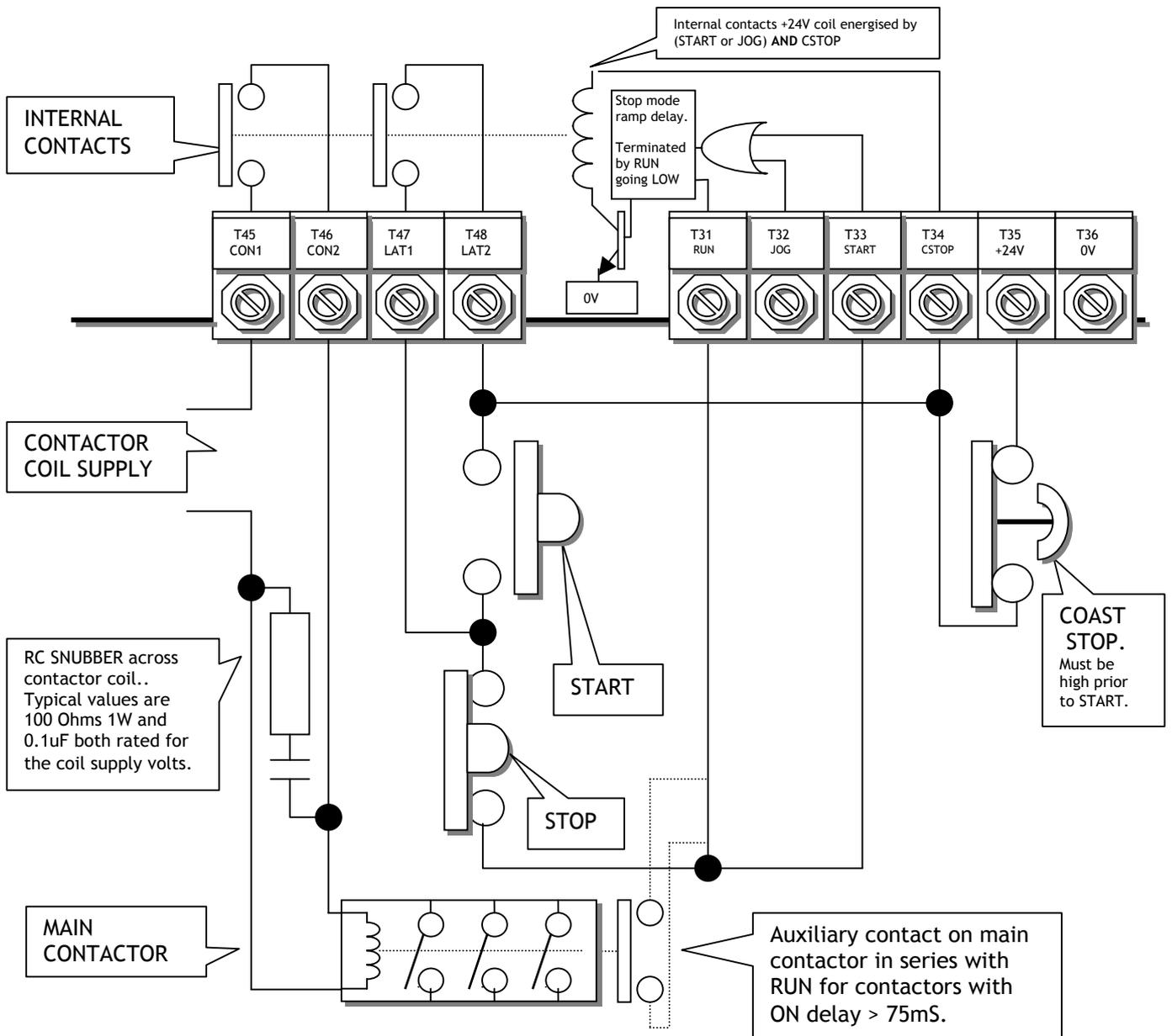
Note. This circuit will cause the contactor to drop out as soon as the STOP button contact is opened because the START input is opened **together with the RUN input**, which over-rides the STOP MODE RAMP function.
