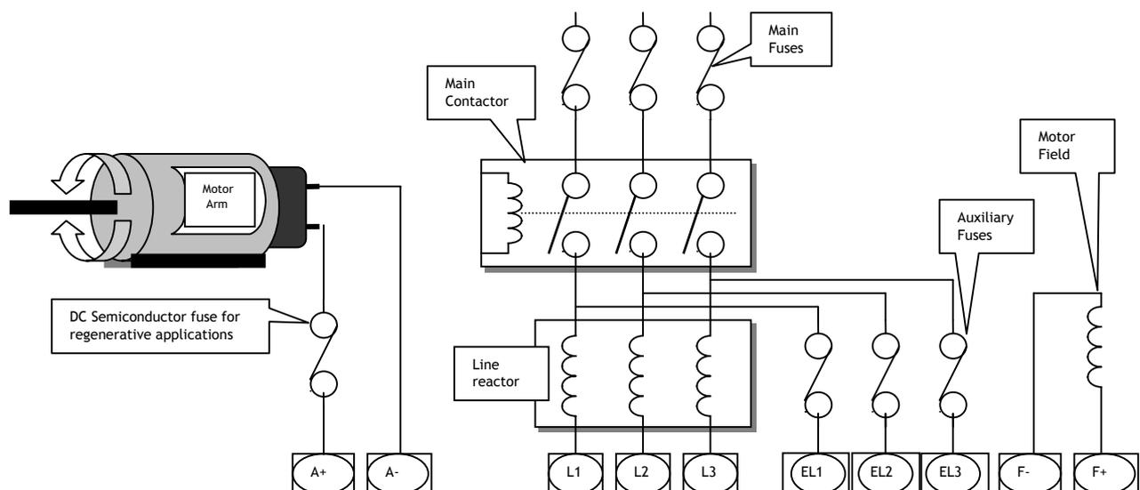
**Advantages** The field winding is electromechanically isolated by the main contactor. Some retro fit installations are only able to provide the 3 main phases because the main contactor is remotely located to the drive panel, in which case this wiring method may be preferred.
