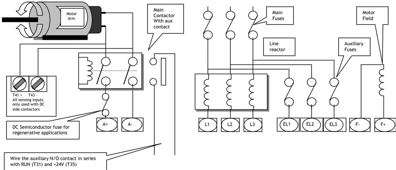
**Advantages** The auxiliary supplies are permanently energised. This allows the synchronisation circuits to lock onto the supply prior to the application of power to the motor. This results in a fast release of current to the armature because it avoids the synchronisation delay. Also the field can remain energised after contactor drop out allowing dynamic braking and/or condensation prevention in standby field mode.
