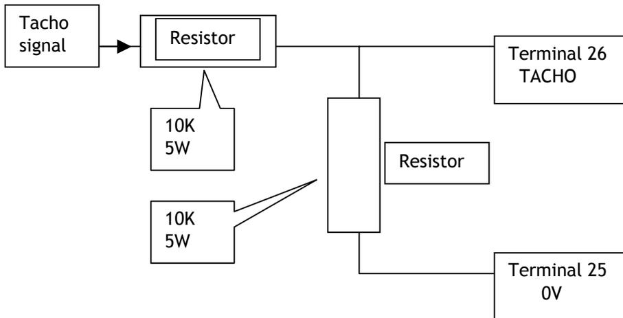
The network shown will allow full scale voltages up to 400 Volts. The number scrolled in the window should be set to half the full scale tacho volts. Appropriate measures must be taken to dissipate the heat from the dropper resistors. The total power in watts dissipated will be  $(\text{Tacho signal volts})^2 / 20,000$ .
