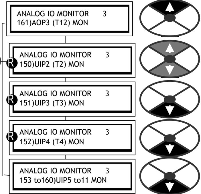
The SPEDESTER possesses a very useful commissioning tool, 260)SCOPE OP SELECT. When enabled, this automatically configures AOP3 on terminal 12 as an oscilloscope probe output. See 13.4.3 ANALOG OUTPUTS / Scope output select PIN 260. The output is automatically connected to whatever parameter is being displayed, and reconnected to its original source after the function is no longer enabled.
