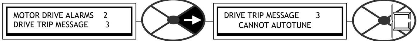
During autotune the drive turns off the field to prevent shaft rotation. An "autotune error" will be triggered by speed feedback being > 20% of rated speed or field current feedback being > 5 % of rated field current during the autotune activity.
