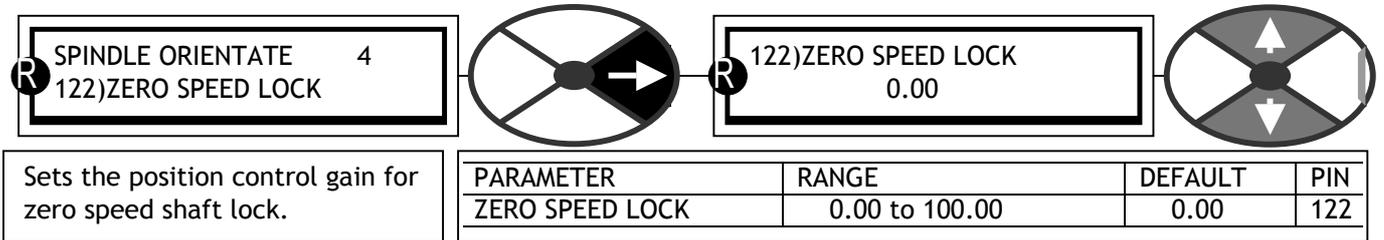
Note, If this value is non-zero, **AND** both speed demand and feedback are less than 117)ZERO INTLCK SPD% an encoder position control loop activates. **The motor must have a bi-directional output shaft encoder. (Quadrature OR pulse and direction).** When locked, the speed may exceed 117)ZERO INTLCK SPD% without losing the lock. Lock is only released by speed demand > 117)ZERO INTLCK SPD%.
