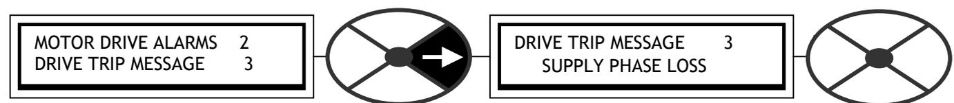
The controller continuously monitors the incoming supply of the EL1, EL2 connections. If either are lost, the alarm will operate. The subsequent control action depends on the running condition at the time the alarm is triggered. The message will also briefly appear after the control supply has been removed.
