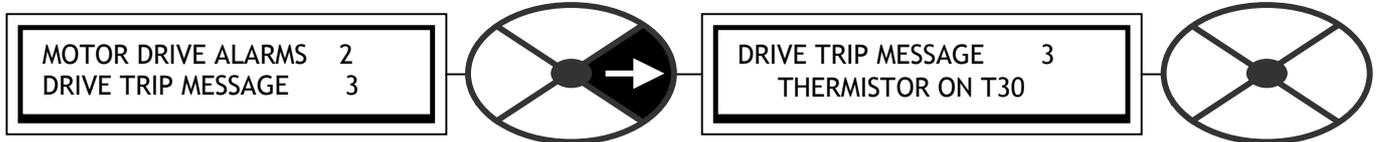
It is good practice to protect DC motors against sustained thermal overloads by fitting temperature sensitive resistors or switches in the field and interpole windings of the machine. Temperature sensitive resistors have a low resistance (typically 200 Ohms) up to a reference temperature (125 deg C). Above this, their resistance rises rapidly to greater than 2000 Ohms. Temperature switches are usually normally closed, opening at about 105 deg C.
