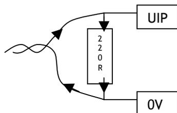
When using 4-20mA loop signals all that is required is to fit an external burden resistor of 220 Ohms between the input and 0V. Then set up the relevant UIP to read the resulting voltage signal generated by passing the signal current through the burden. The diagram shows a 4-20mA signal flowing through an external burden resistor.
