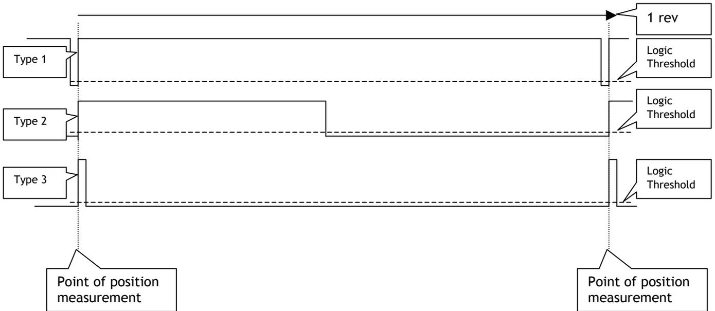
Type 1 is the preferred marker signal. This is because for most of the time the signal is well away from the logic threshold and noise is very unlikely to cause a false marker reading.
