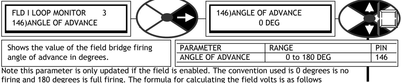
Note this parameter is only updated if the field is enabled. The convention used is 0 degrees is no firing and 180 degrees is full firing. The formula for calculating the field volts is as follows
