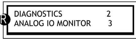
Analogue inputs are UIP2 to UIP9. The UIP number corresponds to its terminal number. (UIP1 is used internally and not available on a terminal). UIP2 to 9 are universal inputs and can be used as digital and/or analogue inputs. The analogue value appears in this menu and the digital logic level will simultaneously appear in the digital IO menu.
