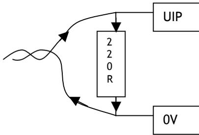
When using 4-20mA loop signals all that is required is to fit an external burden resistor of 220 Ohms between the input and 0V. The resulting voltage signal generated by passing the signal current through the burden will be +0.88V for 4 mA (represents 0%) and 4.4V for 20mA (represents 100%). Using the appropriate UIPX SETUP block, select the following :-
