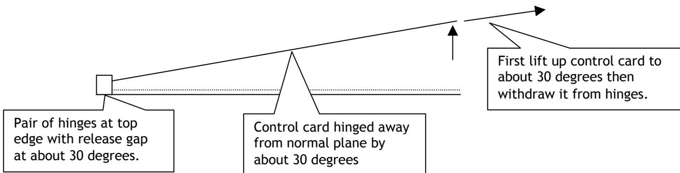
To re-assemble, perform the above procedure in reverse order. The control card is guided by the hinges back onto the interconnect pins. It is not possible to screw the control card flat unless the interconnect pins are all correctly located.
