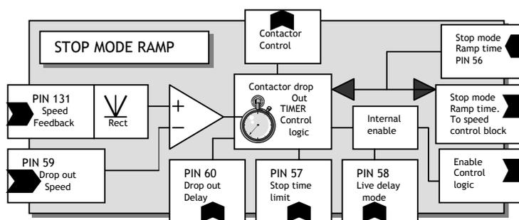
6.5.1.1 Block diagram of contactor control
