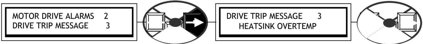
In the event of blower failure, or restriction of the cooling airflow, the heatsink temperature may rise to an unacceptable level. Under these conditions, the heatsink overtemp alarm will operate.
