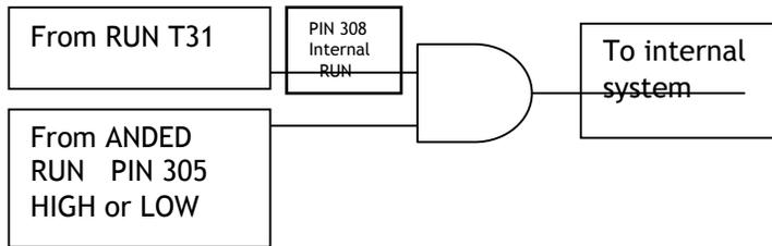
305)ANDED RUN is normally used by a serial link to control the drive. The local hardware terminal in the LOW position will defeat the serial link. The serial link in the OFF position will defeat the local hardware terminal.
