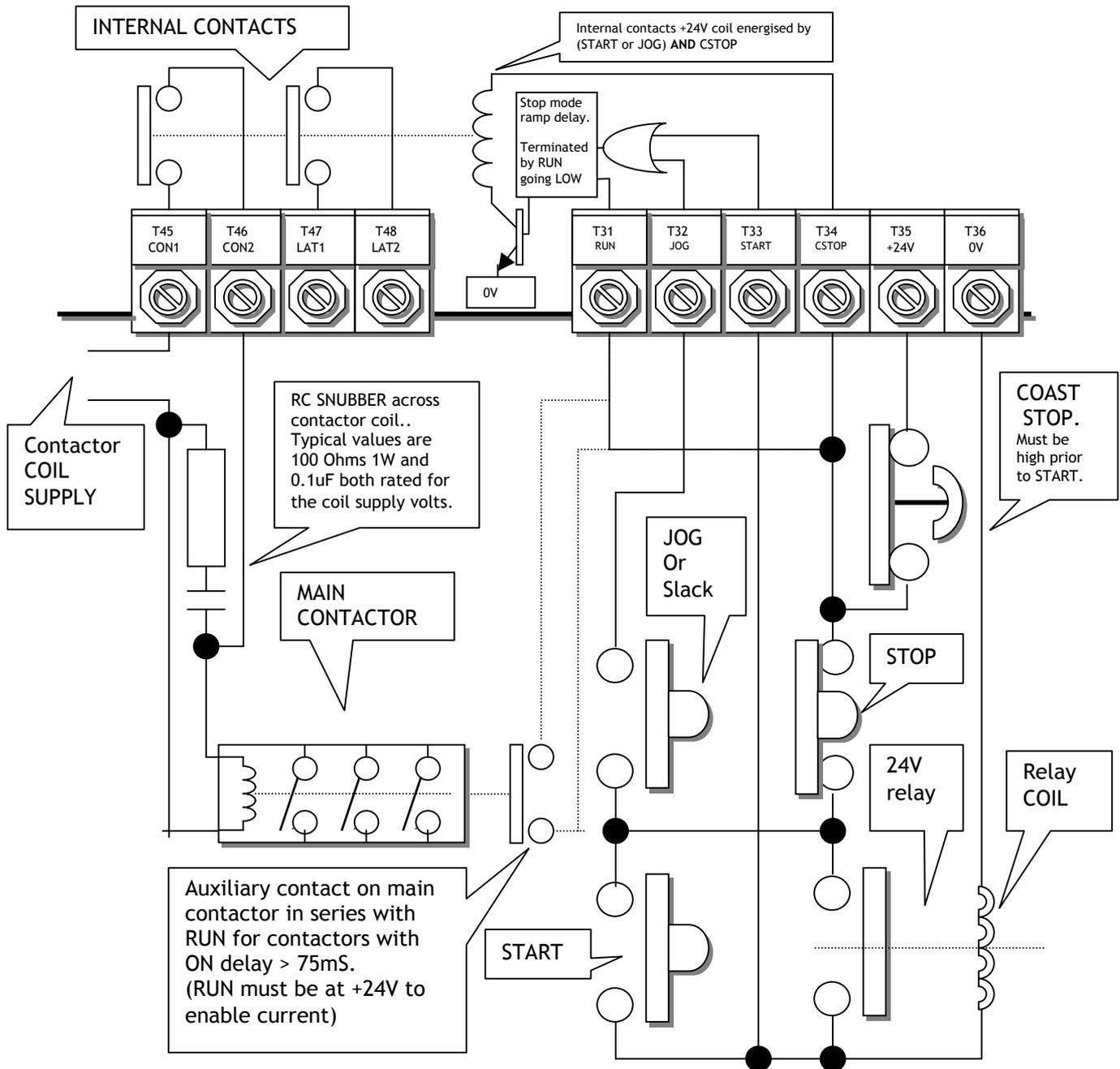
Note. This circuit will cause the STOP MODE RAMP to operate when the STOP button opens during running. Then the speed will ramp down under control of the STOP MODE RAMP. The main contactor will de-energise after the STOP MODE RAMP parameters have been satisfied. See 6.5.1.3 Contactor drop out.
