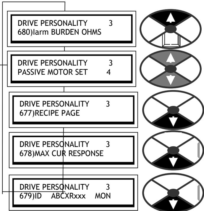
1) **PASSIVE MOTOR SET** contains all the windows used by the **CHANGE PARAMETERS reduced menu** in ascending PIN order to set the passive reduced values for motor 1 or 2.
