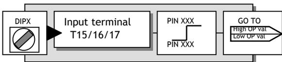
The encoder input type and scaling is programmed by using the CALIBRATION / ENCODER SCALING menu to select the encoder type, sign, encoder lines and rpm.
