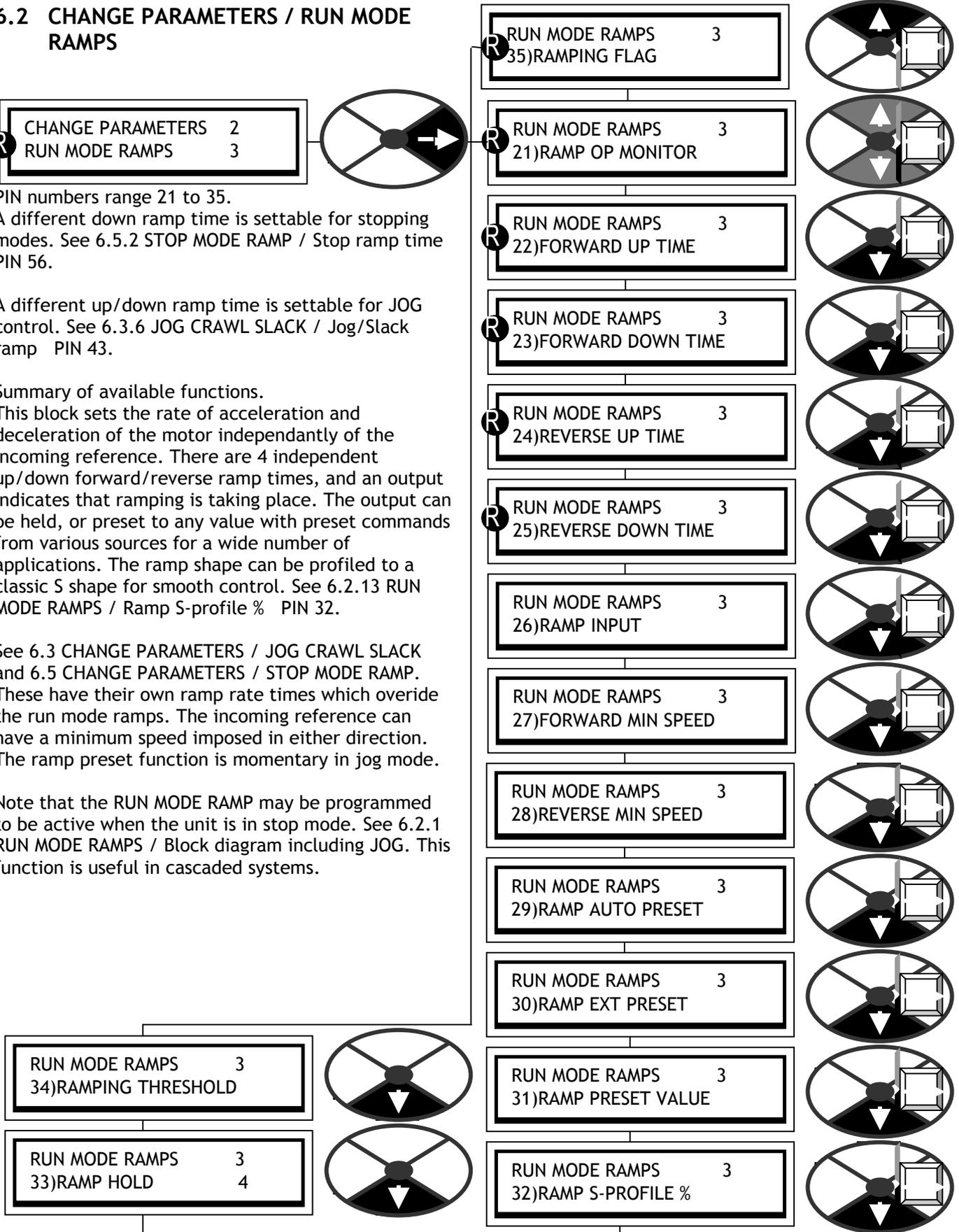
6.2.1 RUN MODE RAMPS / Block diagram including JOG
