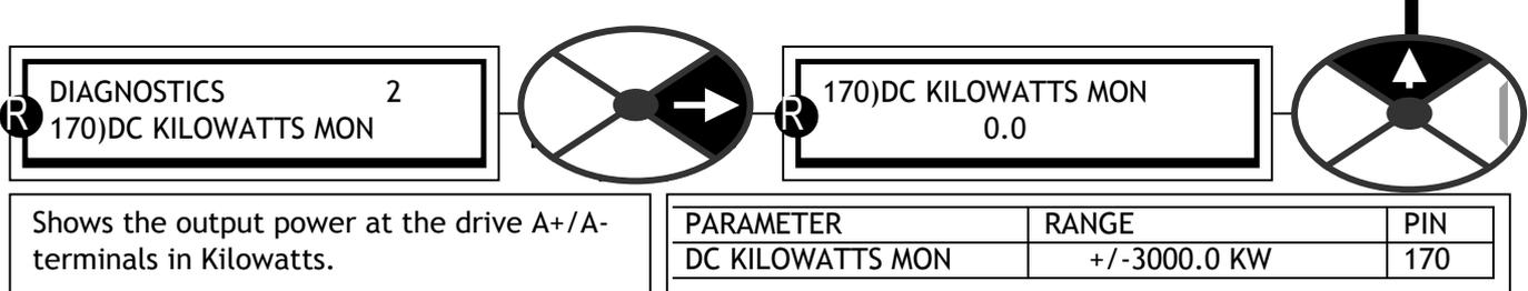
Note. A negative output power shows that the SPEDESTER is regenerating into the AC supply. The power available at the motor shaft will depend on the motor efficiency. (Typically 90 to 95%). To convert Kilowatts to Horsepower multiply by a scaling factor of 1.34.
