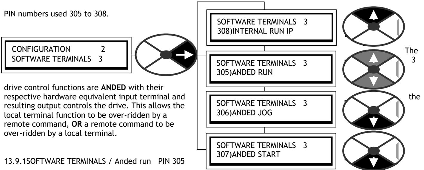
drive control functions are **ANDED** with their respective hardware equivalent input terminal and resulting output controls the drive. This allows the local terminal function to be over-ridden by a remote command, **OR** a remote command to be over-ridden by a local terminal.
