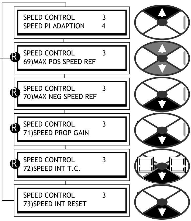
The basic PI gain and time constants are adjustable in this list, and with further sophistication in the sub list SPEED PI ADAPTION. After being output from the error amplifier the signal now represents current reference. This current reference signal is then selected for output by the speed bypass change over switch. If the speed bypass mode is enabled then input reference 3 is selected.
